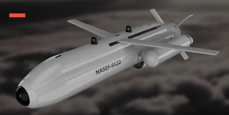
NASEF is a low-cost cruise missile (LCCM) carrying a 50 kg pre-fragmented warhead and with a short to medium flight range capability.
